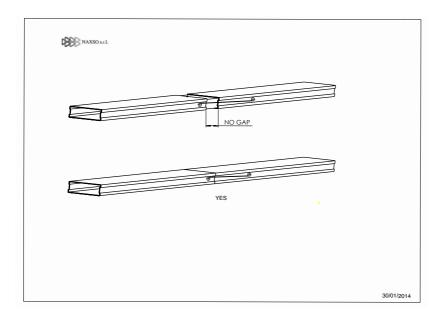
The lighting lenghts shall never be installed flatwise (45mm side face floor) unless a double number of brackets is applied but consider the side 17mm face floor as standard installation. When installing a line be sure the joint screws are face down and screwed and
