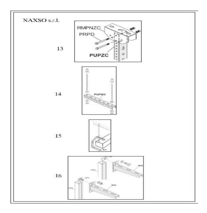
To be sure that the good work made on brackets is useful a strong latching of the busbar to the bracket needs to be assured via all kinds of L and U fixings. As per attached drawings.
