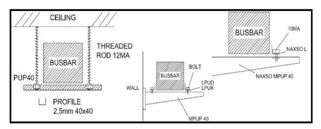
Before lifting the busbars ensure that the lifting procedures can be performed in the area and no barriers are in the path. Fixing brackets have to be placed according to the following minimum requirements:
