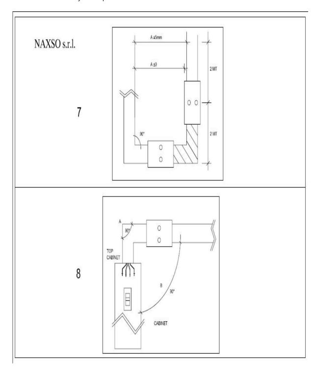
Naxso MPUP and lay the busbar in a stable position thanks to L fixing points like Naxso LPU.
